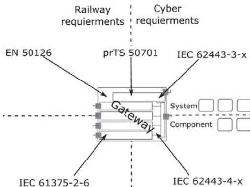
Fig. 1. Certification framework for train cyber gateway.
