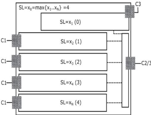
Fig. 2. Diagram of communication channels in the Train Cyber Gateway.
